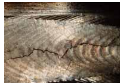
Section Fatigue Crack (50x)
